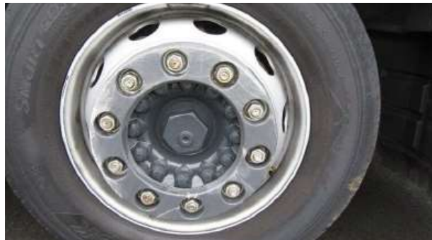
Rims and wheel covers: Multiple superficial scratches with or without removal of material
