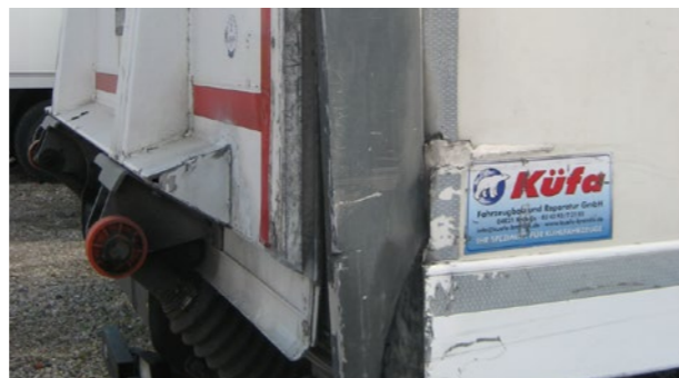
🔧 Side and rear doors: Significant damage: Repair time greater than 1 hr within economic repair, closure not sealed
