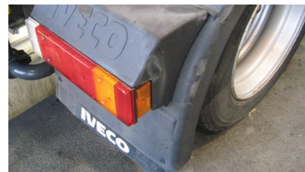
Severe scratches and denting or bending
