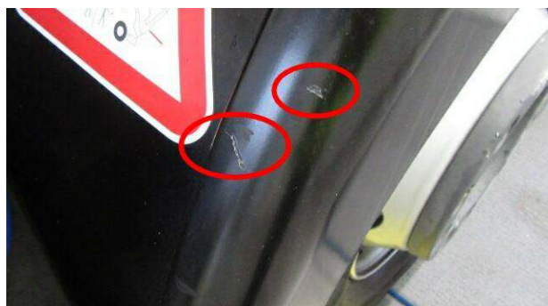
Scratches that cannot be felt with your nail and surface less than 45 cm 2 (equivalent to a credit card)
