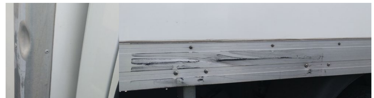
Underbody side profiles: Dents and scratches within economic repair
