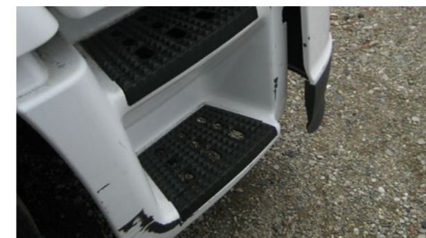
Removal of material, broken part
