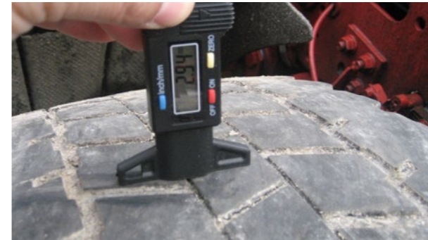
Tyres: Cuts or tears greater than 3mm deep, removal
