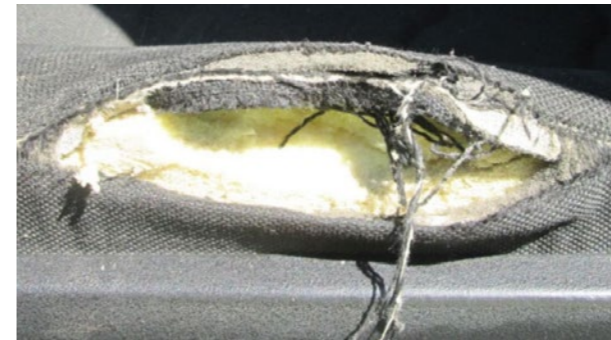
🔄 Foam missing or broken frame
