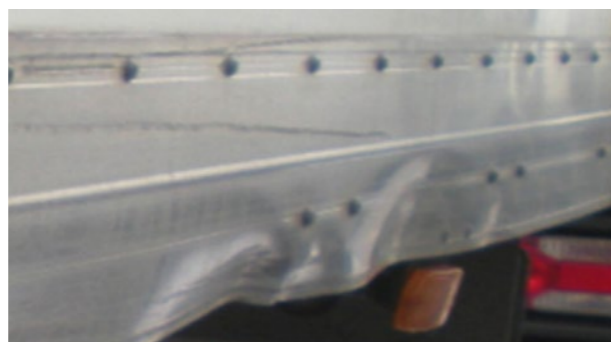
↻ Underbody side profiles: Scratches and dents beyond economic repair, perforations, removal of a section of the profile
