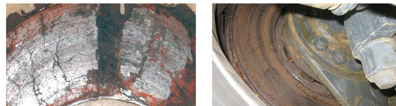
Rusted, ground, worn brake discs
