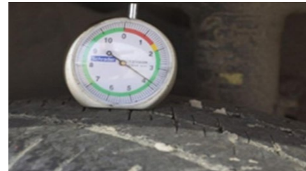
Tyres: Base of groove depth greater than 7 mm Note: The wear of the tyres is measured in the most worn groove on the tyre.
