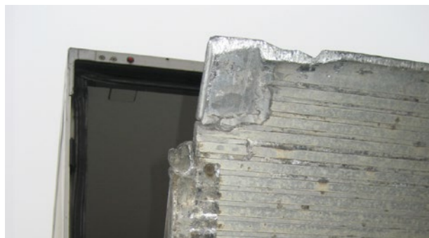
↻ Tail lift: Damage to platform beyond economic repair, broken or incomplete trim
