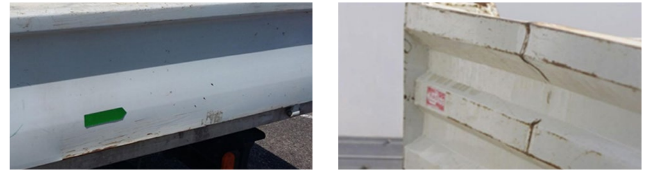
Scratches greater than 20 cm in diameter
