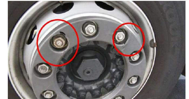
Wheel covers: Twisted, broken, material missing or removed
