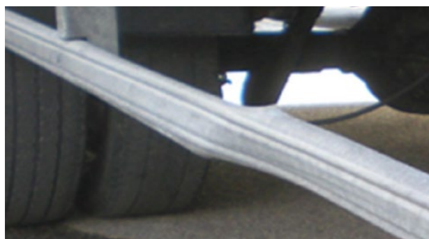
↻ Side Rails: Damage beyond economic repair
