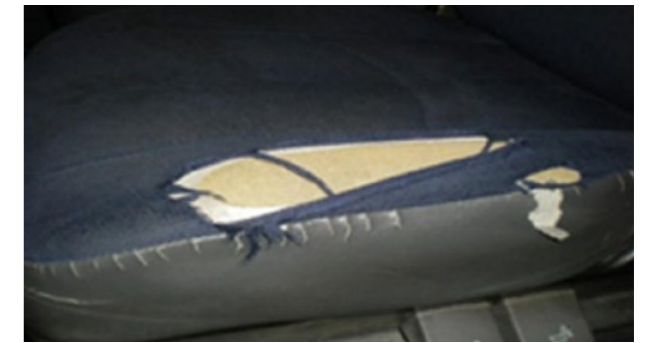
🔄 Burn greater than 3 mm, perforation or tear in the cover, without deterioration of the foam
