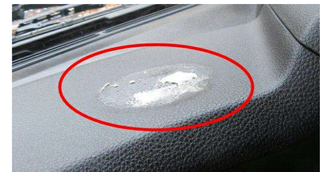
🔄 Fabric and plastic trim: Tear, hole greater than 5 mm diameter, indelible marks
