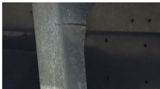
🔧 Tail lift: Damage to platform within economic repair
