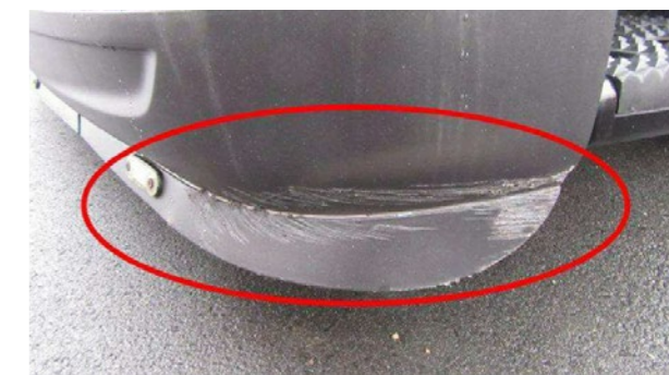
Removal of material or denting feasible or economical to repair
