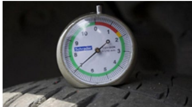
Tyres: Base of groove depth greater than 7 mm (CONFORMS) Note: The wear of the tyres is measured in the most worn groove on the tyre.
