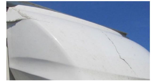
Cabover and deflector: Significant crack, missing part or beyond economic repair
