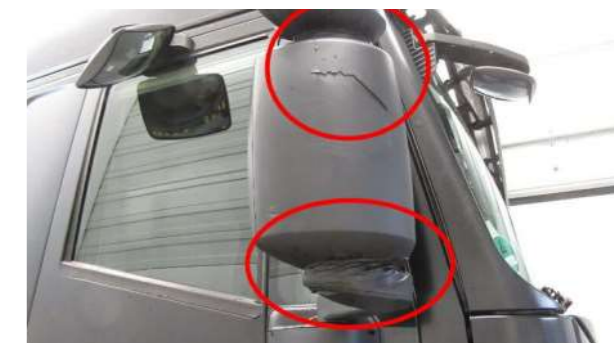
Removal of material or denting feasible or economical to repair
